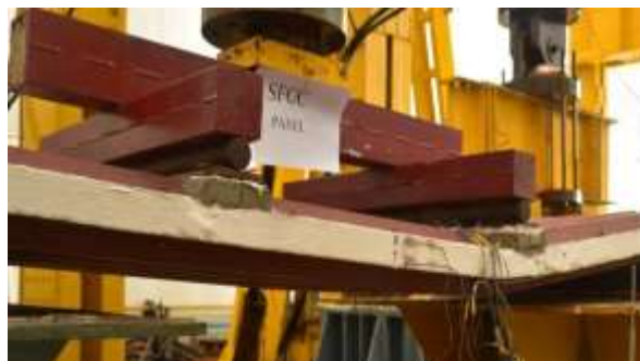
Fig 20 Deflection of SFCC panel 1
