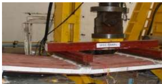
Fig 20 Deflection of SFCC panel 1
