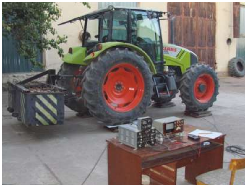
FIGURE 2. Method for determining the vertical forces attributable to the supporting surfaces and taking prints
