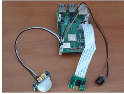
Fig 1. Intruder detection system
