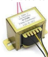
Fig.4 Step down transformer
