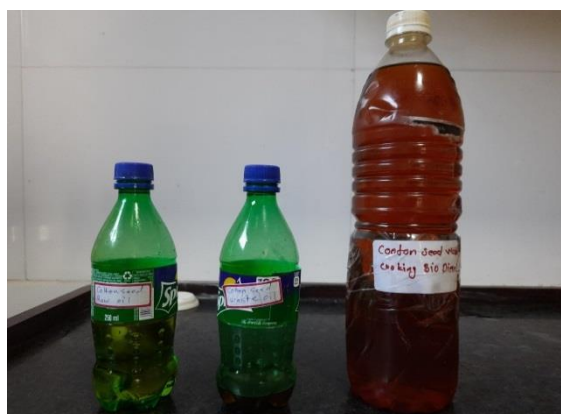
Fig. 2 Raw Cotton Seed Oil, Waste Cooking Cotton Seed Oil and Biodiesel extracted from Waste Cotton Seed Oil
