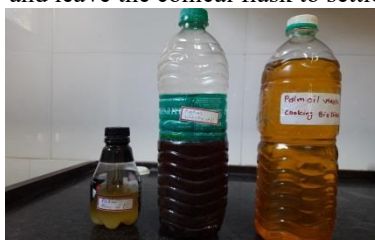
Fig. 1 Raw PAM oil, Waste Cooking PAM oil and Biodiesel extracted from Waste Cooking PAM oil
